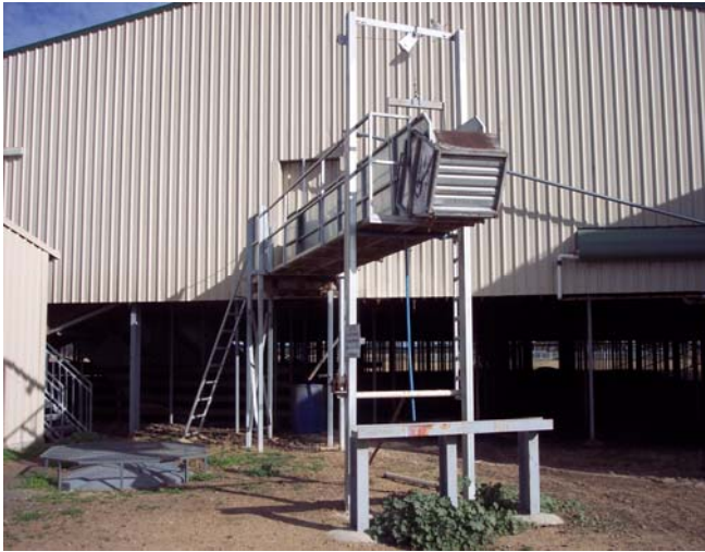
Picture 2: A loading ramp out of a shearing shed provides an adjustable level bridge between the ramp and the float with safety rails to protect the operator. Photograph by G Casburn.
